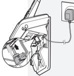
3. Align the grooves on the telephone base with the tabs on the wall mount bracket, and then slide it down until it clicks securely in place.
